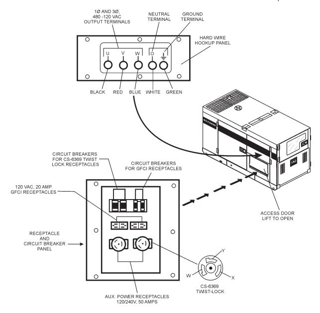
**Figure 8. Output Terminal Panel**
